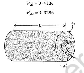
where 1 stands for inner cylinder and 2 stands for outer cylinder.
