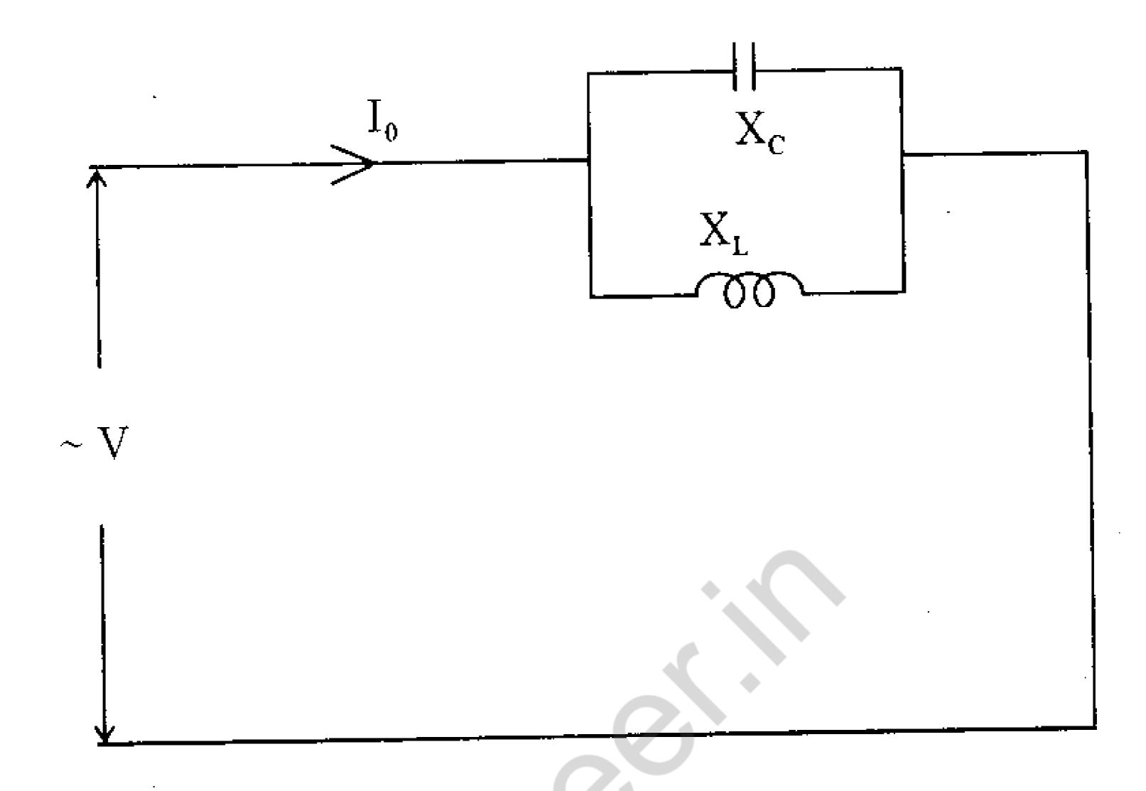
Prove that, under resonant condition, current from source,  $\boldsymbol{I}_0$ , is zero. Assume ideal  $\boldsymbol{X}_C$  and  $\boldsymbol{X}_L$
