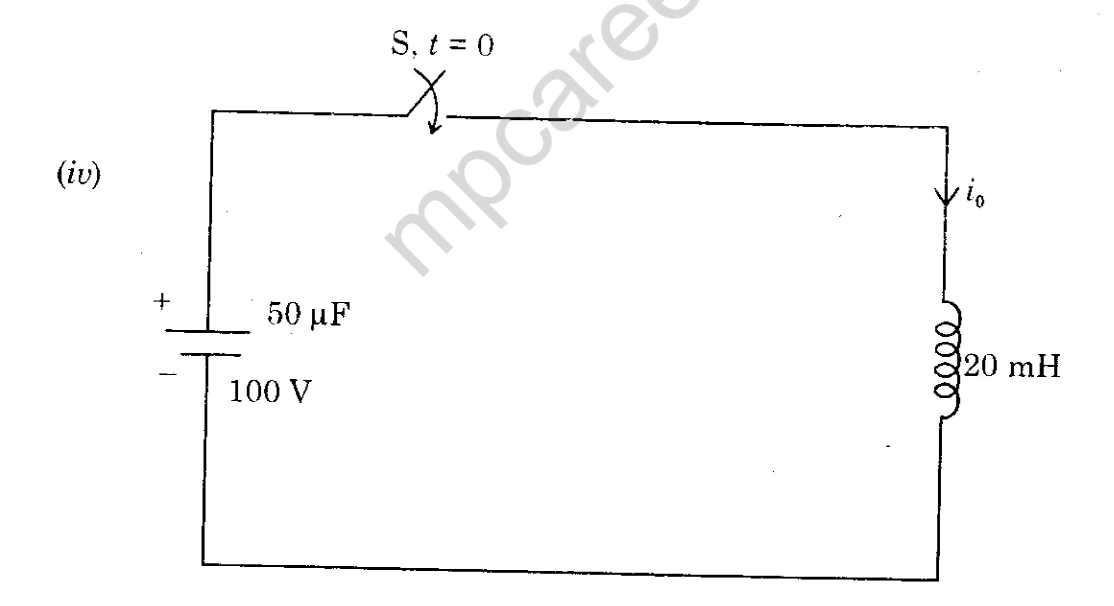
The switch is closed at t = 0. Write the equation of the current  $i_0$ , when the switch is closed at t = 0.
