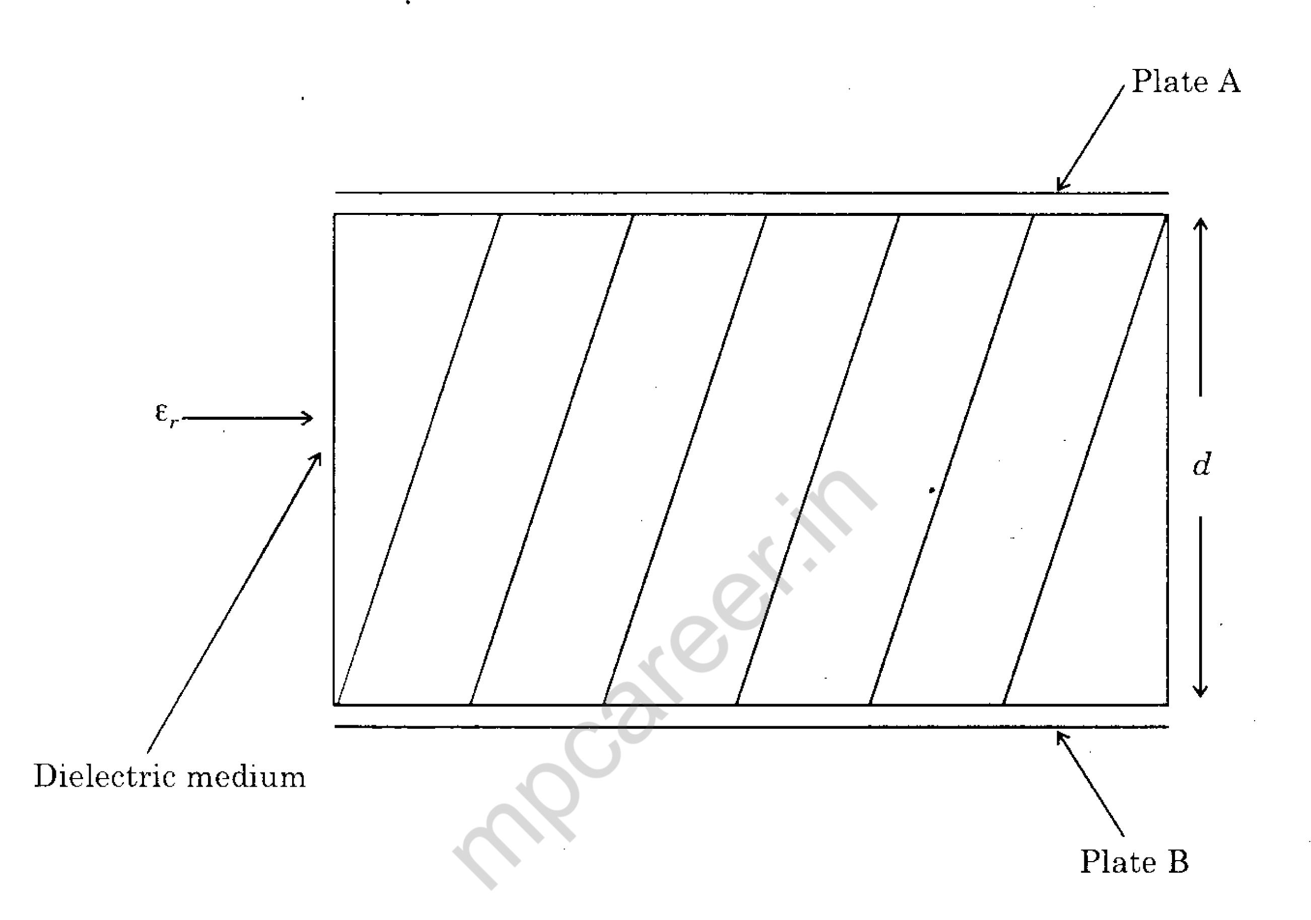
Area of parallel plates is A. Find the equation of capacitane of the capacitor.
