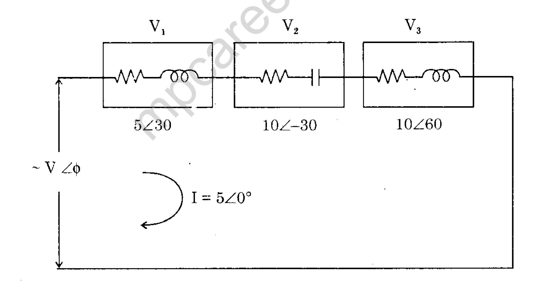
Circuit current is  $I=5\angle 0$  . Calculate  $V_{_1},\ V_{_2},\ V_{_3}$  and  $V\angle \varphi$  and draw phasor diagrams.
